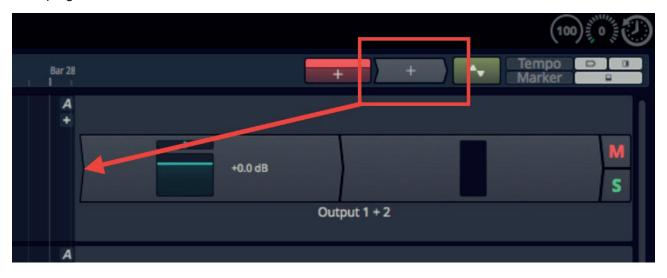
As you hover the icon over the mixer area, you will notice you can place it in any position in the signal chain; any items in the mixer area can be freely moved by dragging at any time. Releasing the icon will bring up the plugin selector menu, where you can locate and select the desired virtual instrument.
